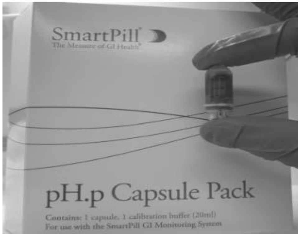
Figure 2: Image of the SmartPill (SmartPill Corporation, Buffalo, NY). The SmartPill is often described as the size of a large multivitamin pill. It measures approximately 1.3 cm by 2.6 cm.
